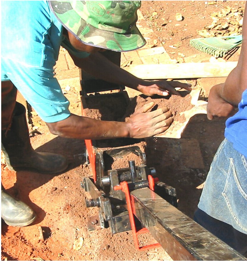
Start filling the brick moulding cavity.
