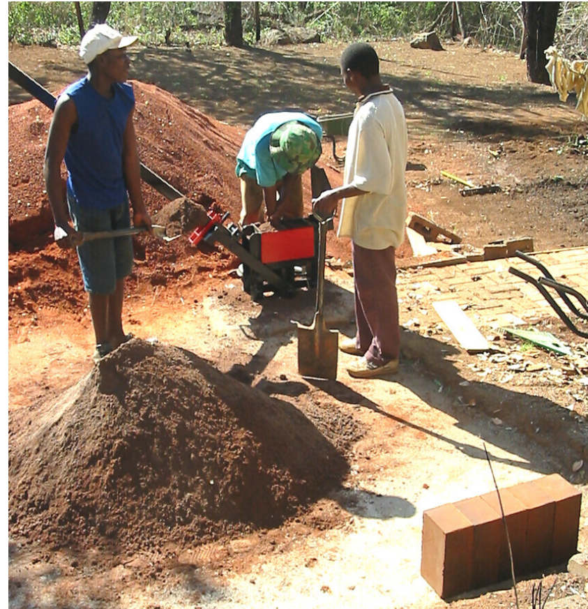
After filling it full, punch the mix down according to the clay content.
